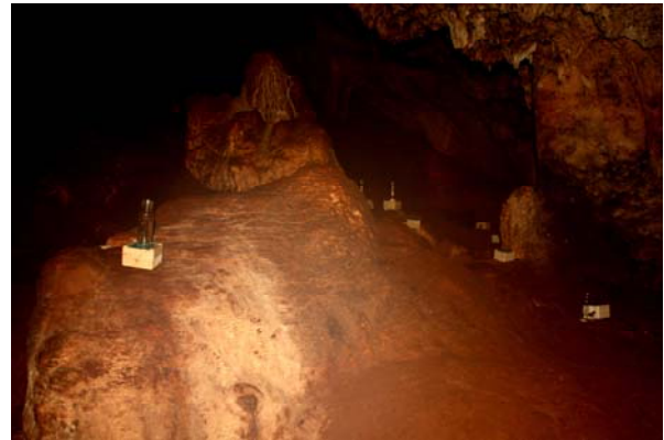
Figure 3. Some of the Stalagmate © drip loggers at Cathedral Cave, Wellington.
